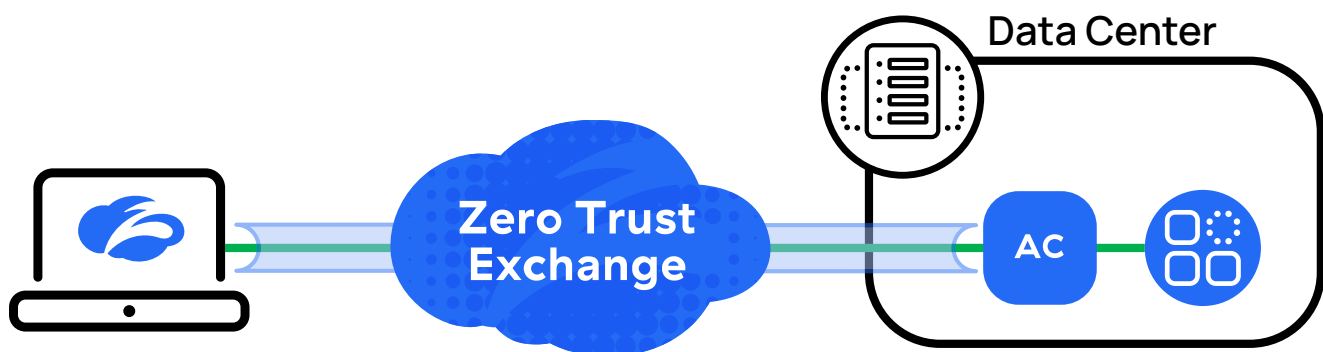
Figure 2. Connections to private applications with ZPA are secured between users and applications
